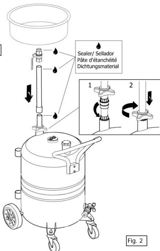
(GB) Assemble the tube with the funnel and fix the assembly on the tank.
